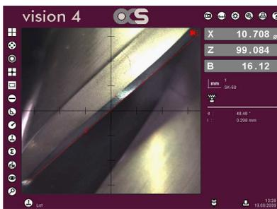
Chamfer width with perpendicular function
